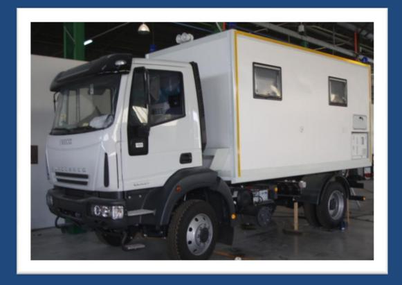
On chassis IVECO ML 100E21W 4x4 rigid-day cab. Equipped with light and acoustic emergency warning and hinged windows.
