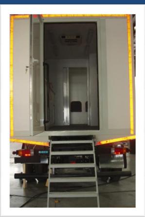
The vehicle composed of two different rooms, that communicate by means of a slinding door. External access to each room is granted by two doors, complete with stairs with no slippery steps. Rear room is dedicated to the sanitary cell, the front instead can be used as an office/waiting room.
