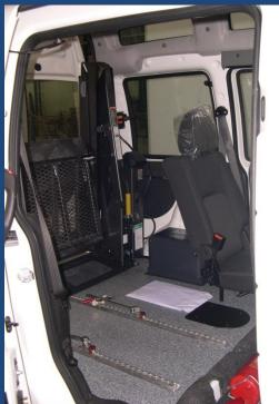
The fitting is complete and includes a single or double lift, seats if required, and rails/fixes and restraining belts.
