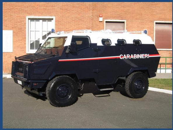
Armoured vehicle, ordinary 7.62 NATO ballistic level on IVECO chassis 40.13 WM 4x4. Crew of seven (plus driver) and/or armament up to a payload of 800 Kg.
